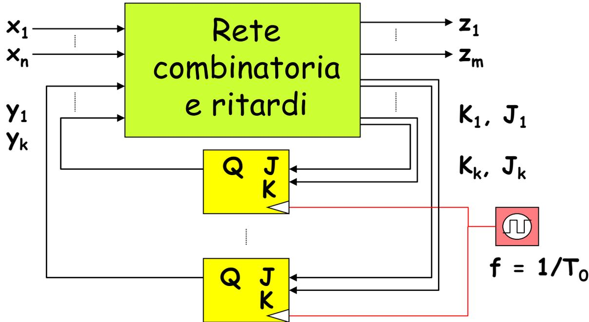
$$z_i^n = F_i(x_1, \dots, x_n, y_1, \dots, y_k)^n \text{ per } i = 1, \dots, m$$
